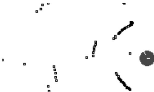
Figure 6.4 Sonar Scan on a Corner
